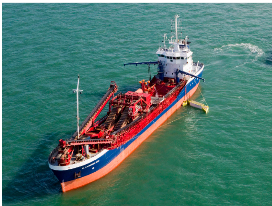
The Vikoseq system has integrated skimmers that are supplied for both high and low capacity requirements.
