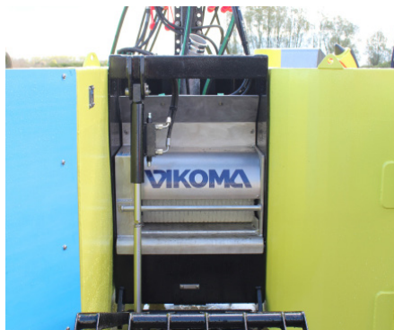
The Vikoseq system has integrated skimmers that are supplied for both high and low capacity requirements.
