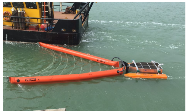
Above: Fasflo operating as a side sweep on a vessel of opportunity
