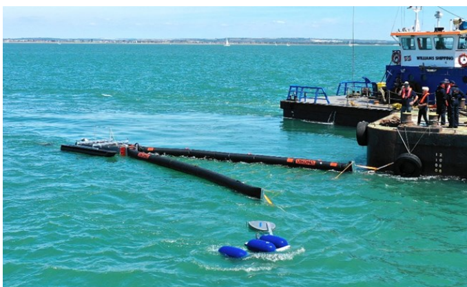
Above: Fasflo Maxi skimmer with Paravane Maxi replacing a tow boat
