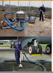
A lightweight, hand portable vacuum recovery system for oil spill clean up
