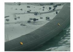
Complete with a galvanised, long link ballast chain in skirt pocket, providing high tensile strength with good underwater profile to ensure maximum oil retention. The skirt is fitted with vent holes to ensure effective drainage.
