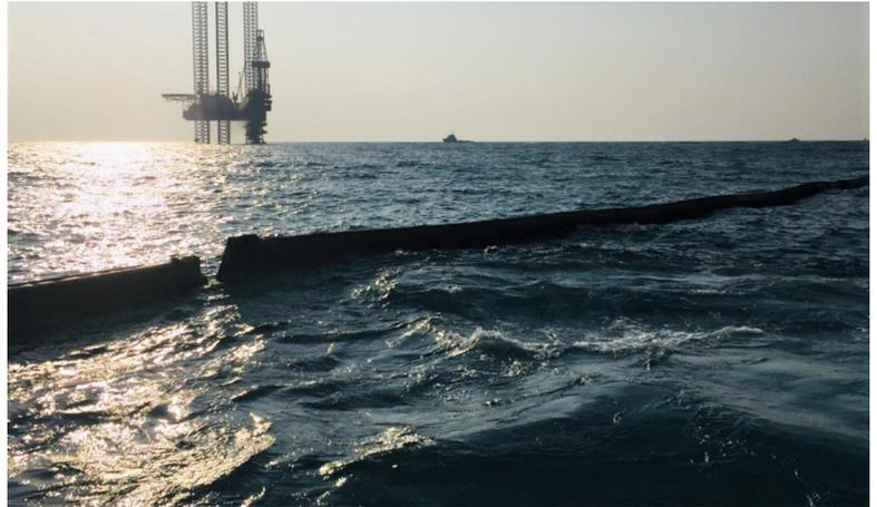
*Hi Sprint boom containing oil in a spill*
