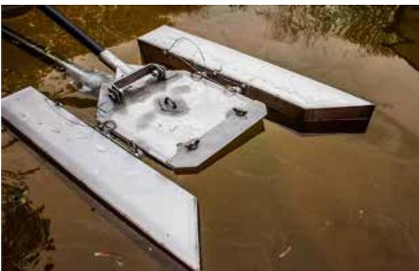
Crust Lance floating suction head in operation
