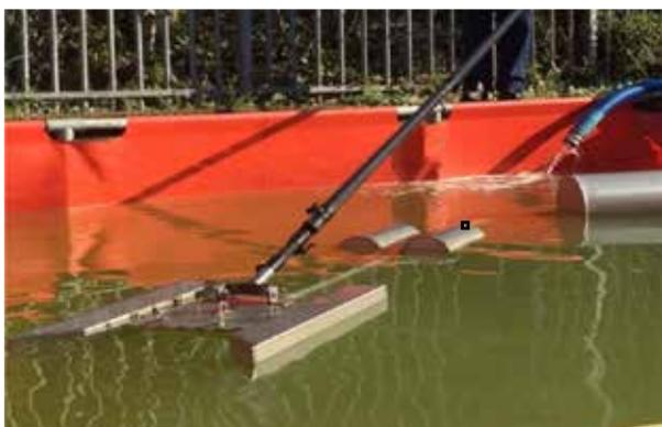
Operator manoeuvring the suction head to recover crust
