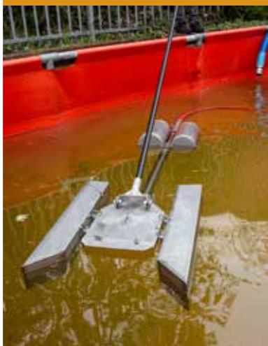
A skimmer for recovering crust forming hydrocarbons from wastewater in tanks, waste pits and separators
