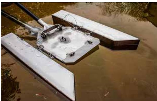
Crust Lance floating suction head in operation
