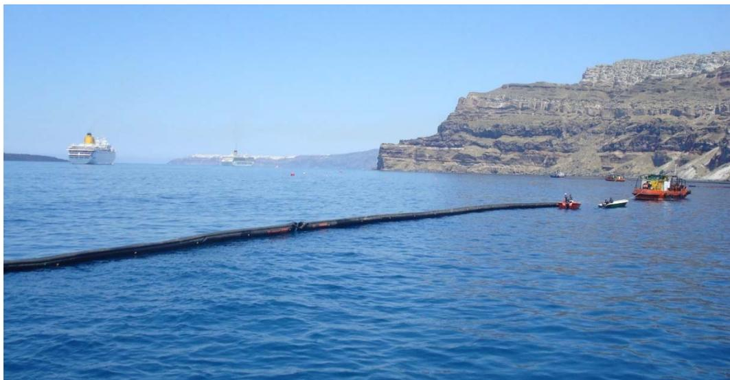
*Left: Hi sprint boom being deployed, quickly with single point inflation*
