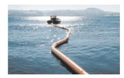
Sentinel boom can also be supplied with closed cell foam filling to provide a permanent or semi permanent boom ideal for protection of water intakes and high risk areas in ports and harbours.
