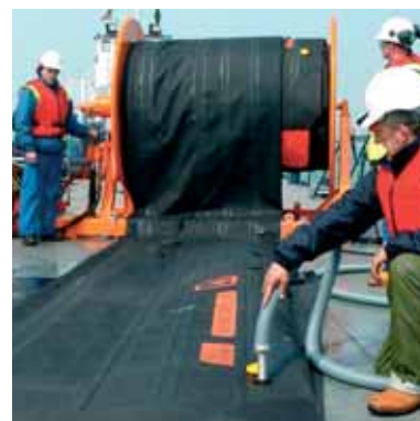
ONE YELLOW CAPPED DEFLATION VALVE PER CHAMBER POSITIONED ON EXTERNAL BOOM SURFACE
